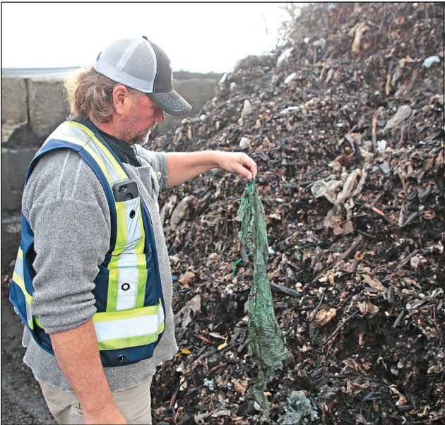
PHOTOS BY MARC KITTERINGHAM Jack Vanderbasch pulls the remnants of a biodegradable plastic bag from the pile after it spent months in the composting process at Coast Environmental’s facility in Chemainus.
