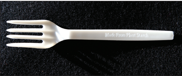
An innocuous fork made from plant starch before (above) and then virtually unchanged after it spent months in a high-temperature composting environment in Chemainus (below).
