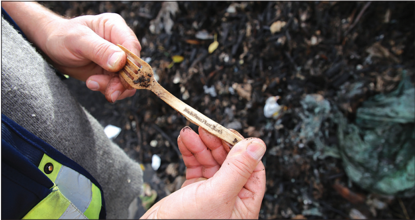
An innocuous fork made from plant starch before (above) and then virtually unchanged after it spent months in a high-temperature composting environment in Chemainus (below).
